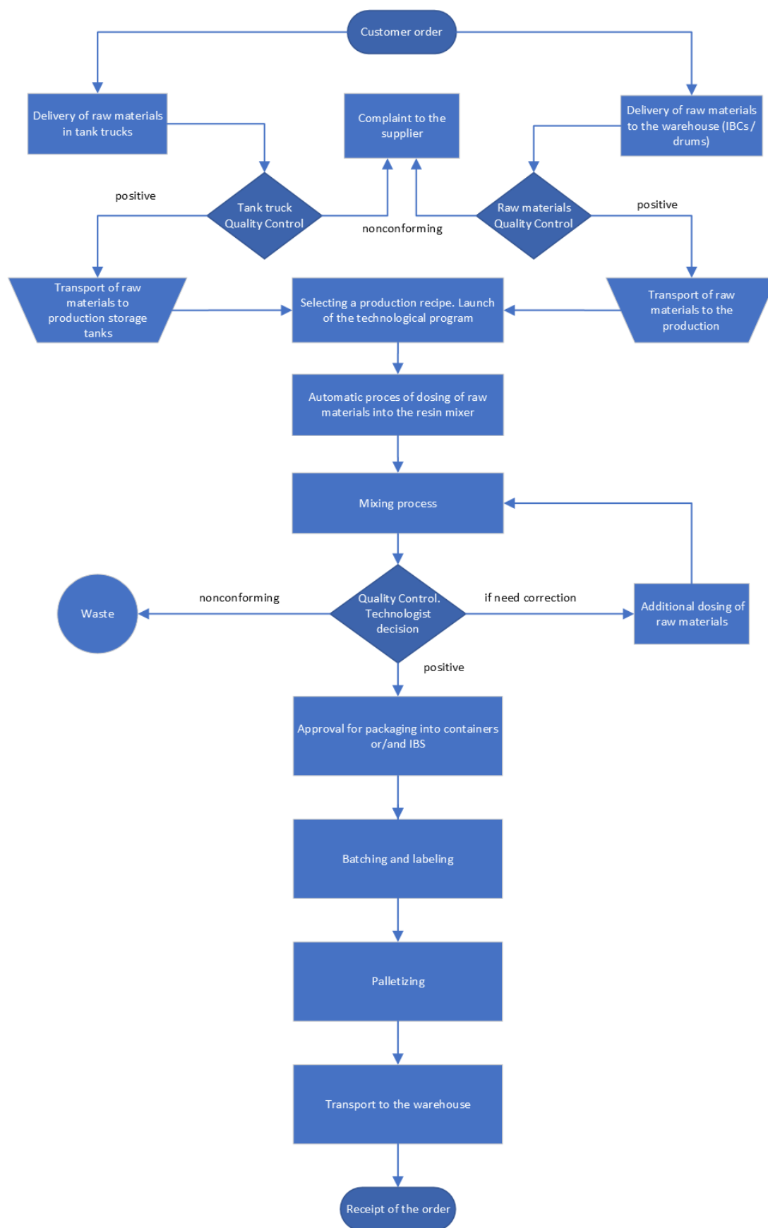
Figure 3. The scheme of injection silicate resins industrial process conducted by DSI Schaum Chemie Sp. z o.o.
