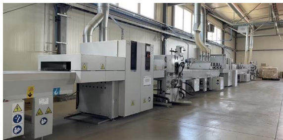
Fig. 1 Production line for UV oiling and varnishing (left) and a line for profiling floors (right) of Podłogi Sp. z o.o. production plant located in Łańcut (Poland).
