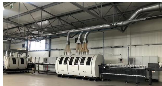
Fig. 1 Production line for UV oiling and varnishing (left) and a line for profiling floors (right) of Podłogi Sp. z o.o. production plant located in Łańcut (Poland).
